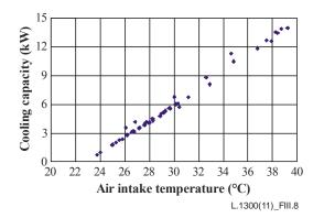
Figure III.8 – Air intake temperature and cooling performance
