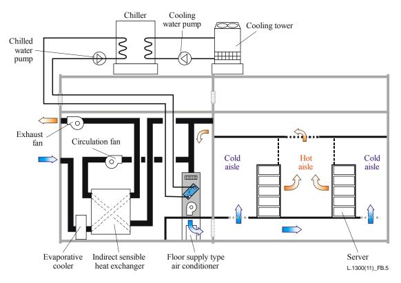
Figure B.5 – Outline of an evaporative cooling system
