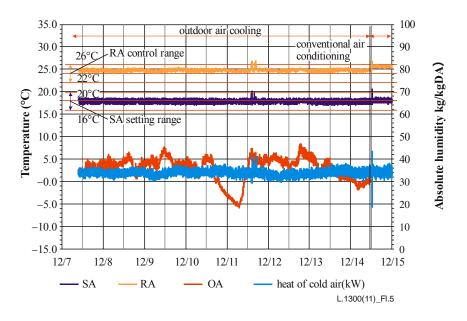
Figure I.5 – Air (SA, RA, OA) temperature and heat energy
