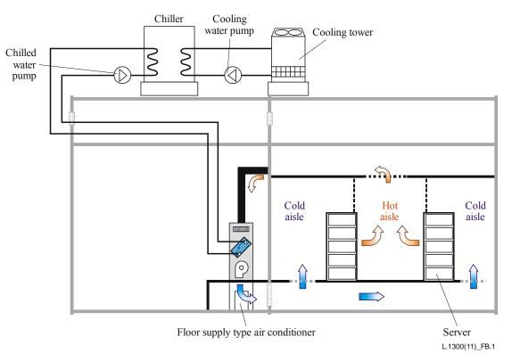
Figure B.1 – Conventional air conditioning system
