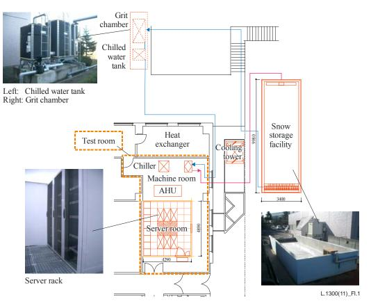
Figure I.1 – Layout of the test facility
