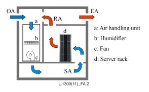
Figure A.2 – Direct use of outdoor air for cooling
