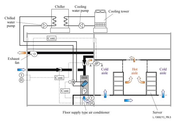
Figure B.3 – Outline of an outdoor air cooling system
