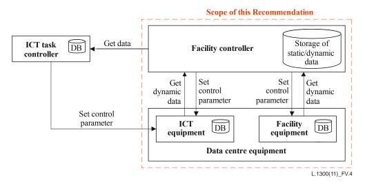
Figure V.4 – Example of control architecture
