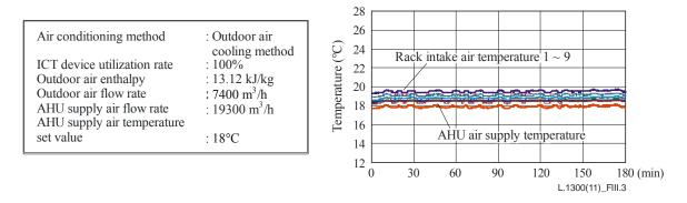
Figure III.3 – Example of air conditioning in an outdoor air cooling system
