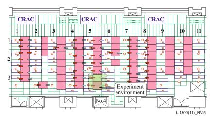
Figure IV.5 – Layout of experiment room
