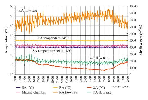
Figure I.6 – Air temperature and airflow rate
