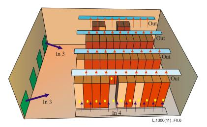
Figure II.6 – Schema of air distribution in scenarios 3 and 4
