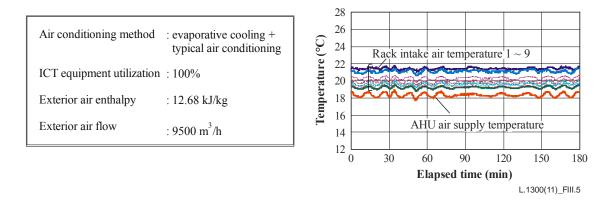
**Figure III.5 – Evaporative cooling operational state (example)**
