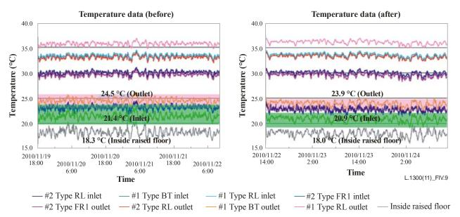
Figure IV.9 - Results of Rack 1 after installing a duct at the outlet and at the inlet
