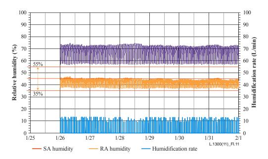
Figure I.11 – Relative humidity of air and the humidification rate
