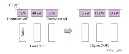
Figure V.2 – Illustration of a server room (COP: coefficient of performance)
