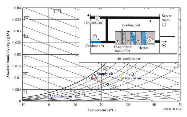
Figure B.4 – Air status in an outdoor air evaporative cooling system
