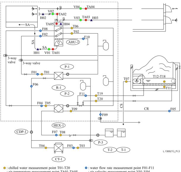
• : air temperature measurement point TA01-TA05 : air humidity measurement point H01-H04
