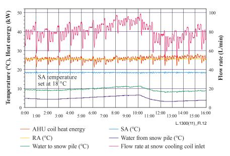
Figure I.12 – Air temperature in snow and ice cooling
