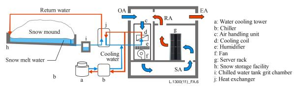
Figure A.6 – Equipment with hybrid cooling facilities
