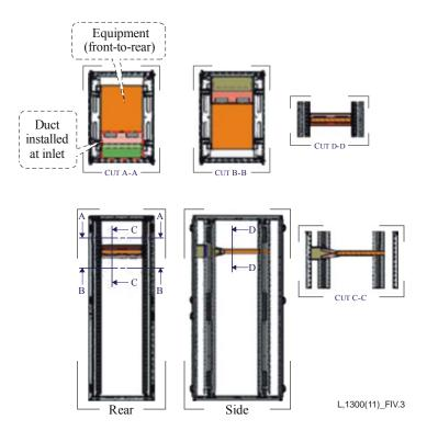
Figure IV.3 – Example of duct installation in equipment that is small in depth
