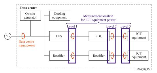
Figure V.1 – Example of a power feeding system of a data centre
