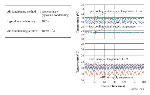
Figure III.7 – Spot cooling method operational state (example)
