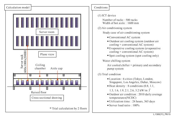
Figure III.10 – Calculation model and condition
