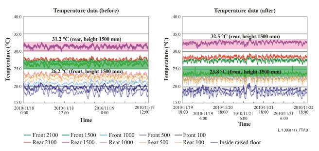
Figure IV.8 – Results of Rack 1 after installing a duct at the outlet
