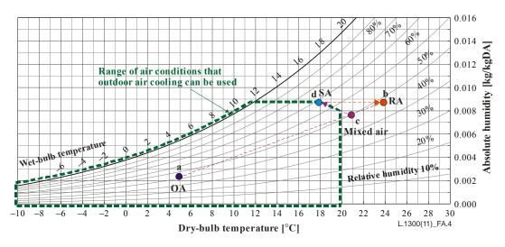
Figure A.4 – Changes in air condition during outdoor air cooling
