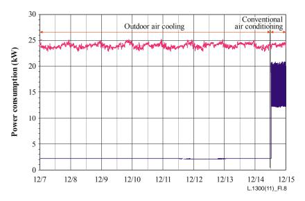
Figure I.8 – Power consumption of servers and air conditioning equipment
