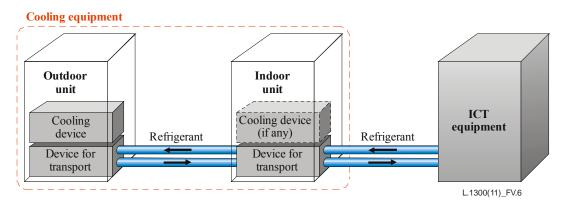
Figure V.6 – General configuration of cooling equipment
