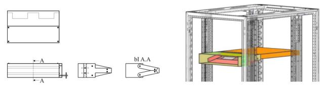
Design of the duct (left) and image of duct installation to the equipment (right)
