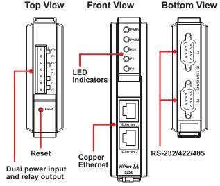
**Reset Button**—Press the *Reset button* continuously for 5 sec to load factory defaults: Use a pointed object, such as a straightened paper clip or toothpick, to press the reset button. This will cause the Ready LED to blink on and off. The factory defaults will be loaded once the Ready LED stops blinking (after about 5 seconds). At this point, you should release the reset button.
