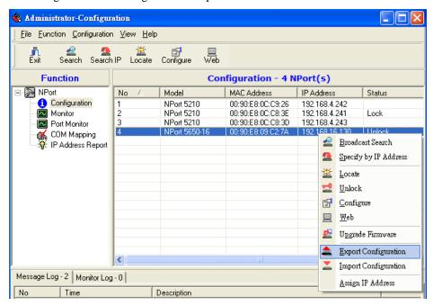
2. The Import Configuration function is used to import an NPort configuration from a file into one or more of the same model NPort.
