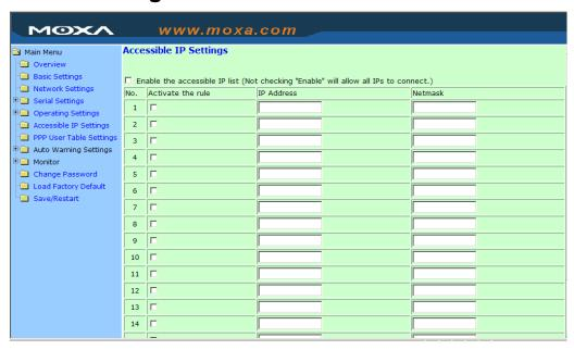
NPort has an IP address based filtering method to control access to itself.
